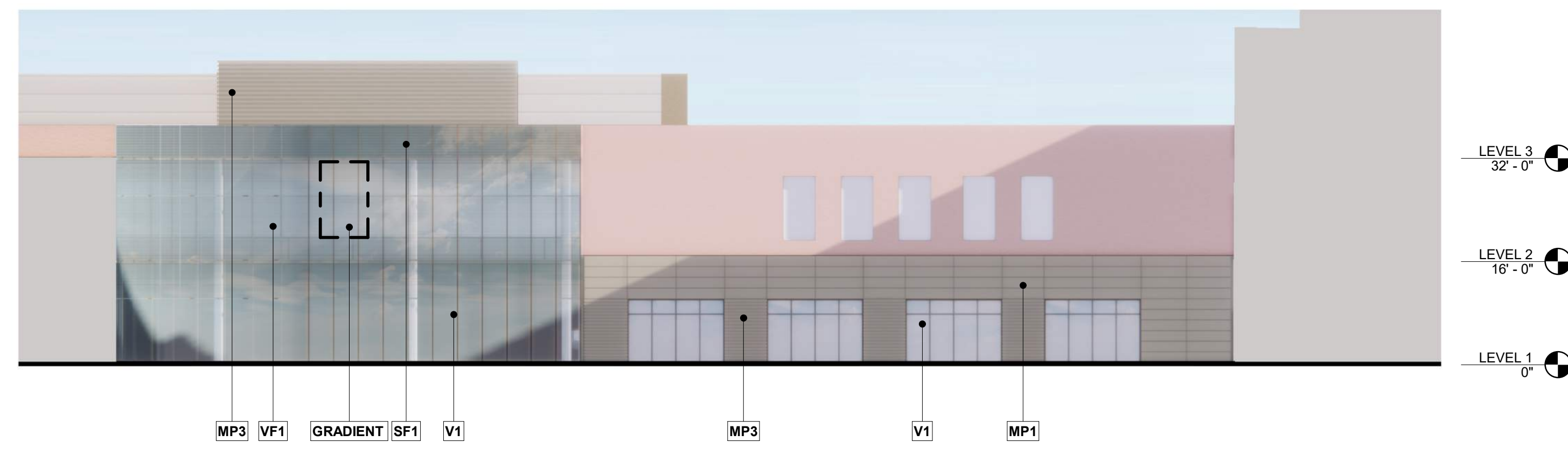
4 COMPOSITE BUILDING ELEVATION - WEST 2 1/16" = 1'-0"
