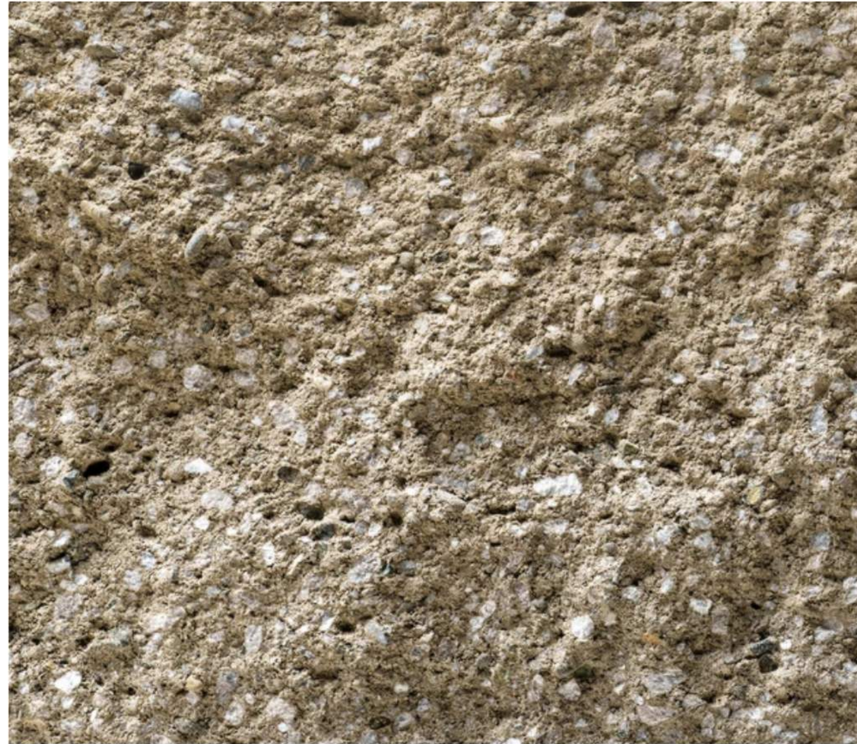
CMU1 SPLITFACE CMU (BASALITE CONCRETE)
