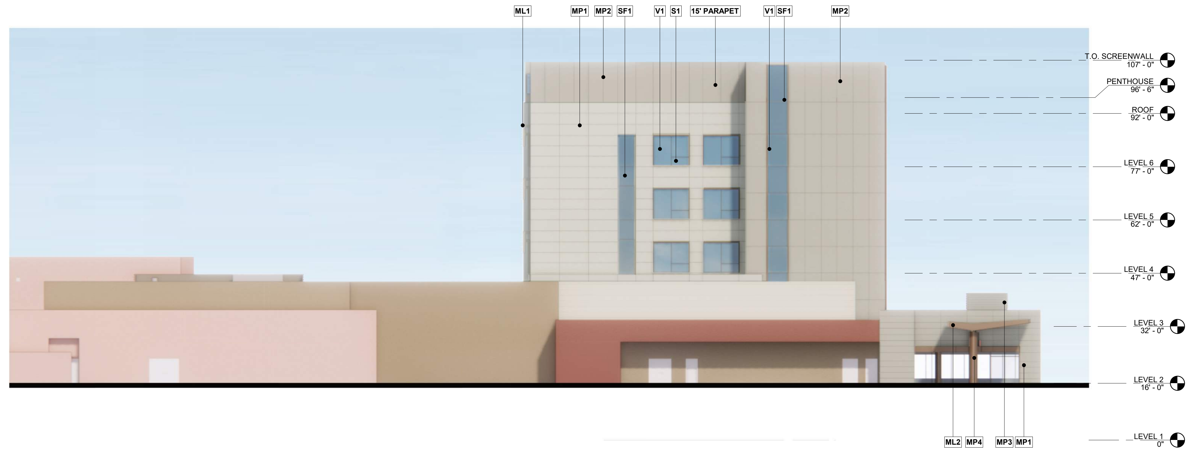
2 COMPOSITE BUILDING ELEVATION - EAST 2 1/16" = 1'-0"
